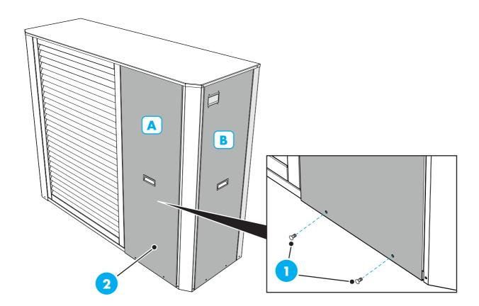
disengage the panel (2) by sliding it downwards (C);
