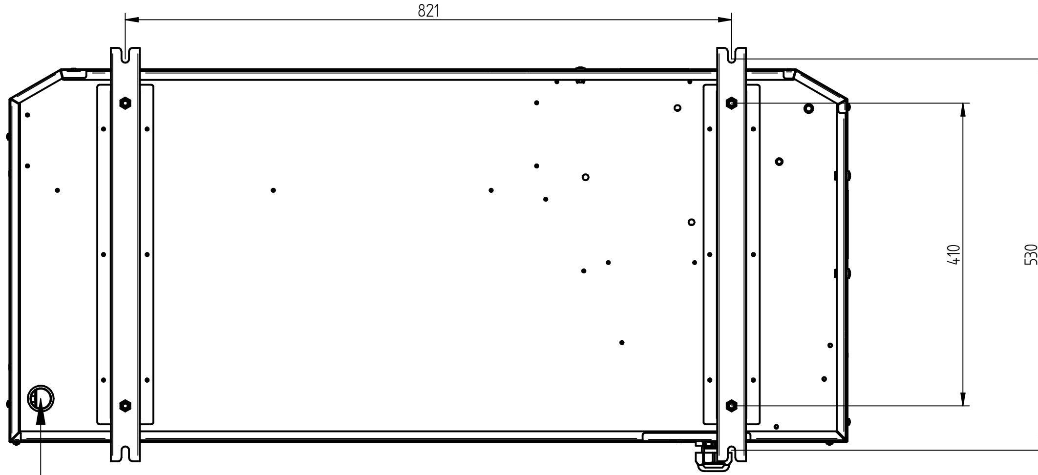
SCARICO CONDENSA  $\Phi i$  27 mm
